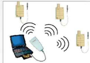
Typical ULP network controlled by a GPort connected to a notebook PC
